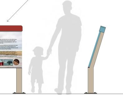
Outfitted with pressure-treated wood posts, galvanized end-caps on top, and substantial metal sleeve-footing (into concrete). Sign faces are full color, high pressure phenolic laminate panels. "Tillamook Coast Experience" medallions are bronze-tone, stained and sealed.
